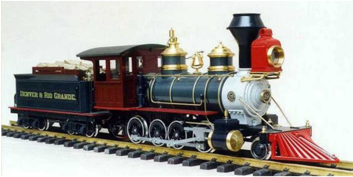
The stunning production model of the Delton C-16, D&RG 1880s Class 60 2-8-0, as delivered to the market in 1989. (Photo D. Fletcher).
