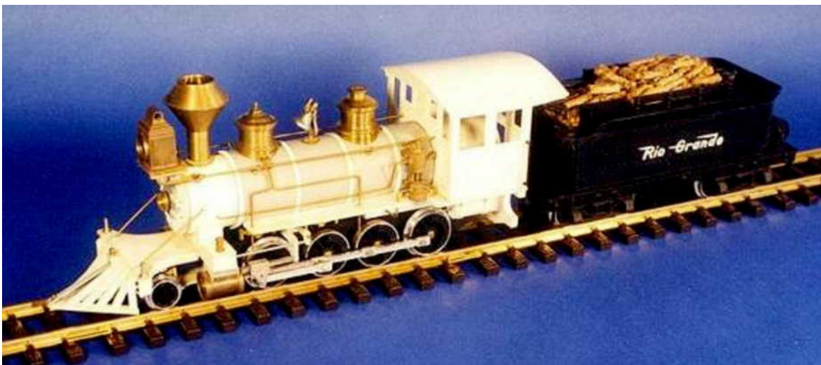
A view of Phil Jensen's hand made, as yet unpainted pre-production model of the famous Delton C-16, 1986, note the construction method used, including brass castings, styrene and PVC.
