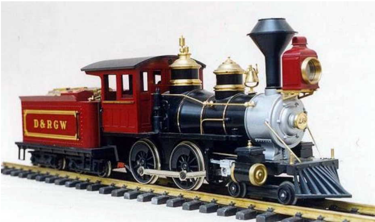
One of the handful of updated 4-4-0s produced by Kalamazoo in 1991, involving the many changes developed by Phil Jensen. Note the use of the Delton C-16 headlight, domes, steam chest covers, air compressor and cab. A huge improvement over the original Kalamazoo 4-4-0 of 1980. (Photo D. Fletcher).
