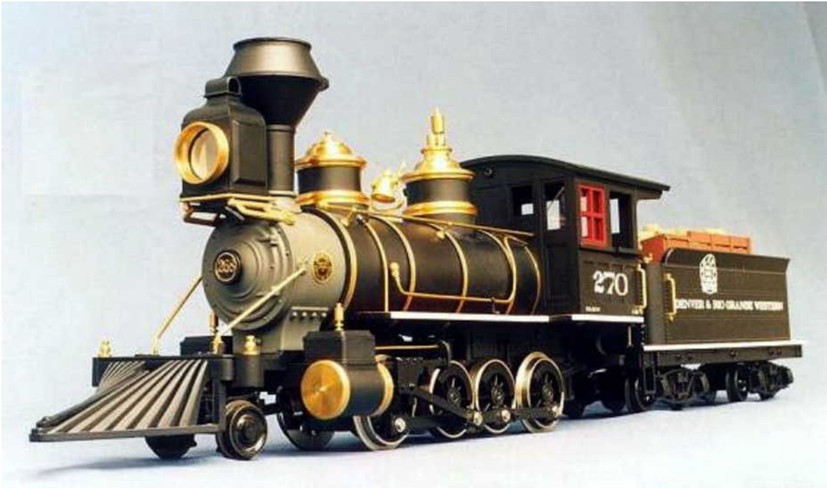
The Delton C-16 hits the market again in 1999, with some replacement tooling, a totally redesigned chassis, and drive mechanism and a host of new paint schemes. (Photo D. Fletcher).
